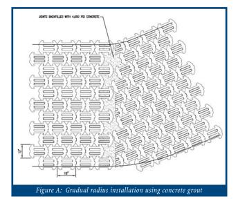
to side, therefore, making them unable to be laid on a radius. If the soil grade is greater than 4:1, it is best to begin placing units at the toe of the slope.
